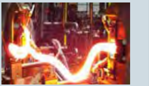
Example of electrification of heat treatment: "Electric heating of stabilizer bars"
