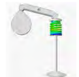
Computer simulation to visualize the behavior of valve springs when driven at high speeds
