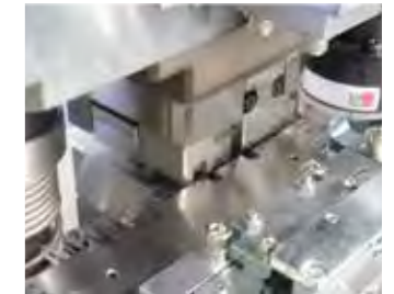
Stamping process for HDD suspensions using high-precision dies
