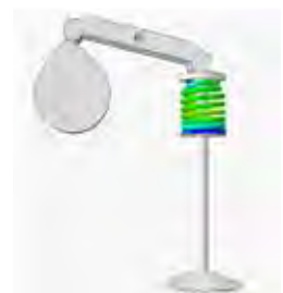
Computer simulation to visualize the behavior of valve springs when driven at high speeds
