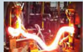
Example of electrification of heat treatment: "Electric heating of stabilizer bars"
