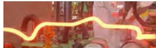
Electric current heating for stabilizer bar [Reduces CO 2 emissions]
