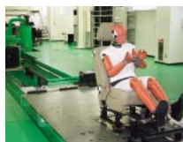
New hydraulic sled testing device
