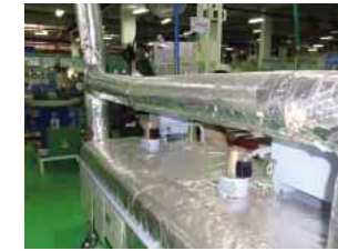
Furnace insulation cover that raise the thermal retention of the furnace (NHK Spring, Thailand)
