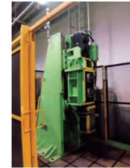
Electric servomechanism fatigue testing machine
