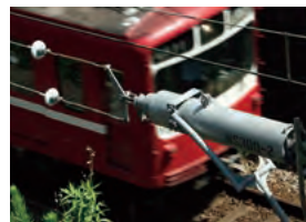
12 Tension balancers for railway use This device uses springs to maintain fixed tension in railroad overhead lines.
