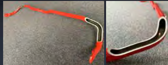
Hollow stabilizer bars Meeting the need for weight reduction, an essential factor in improving fuel efficiency, with processing technology that uses high-strength hollow tubes
