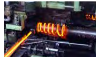
Coil spring forming by NC coiling machine
