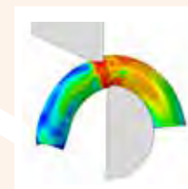
Stress distribution during coil spring cutting [Processing analysis]
