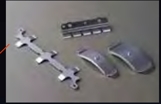
Leaf springs for cooling HEV and EV elements These spring hold semiconductors to heat sink with the force of spring.
