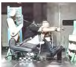
Safety evaluation for seats through hydraulic sled tests
