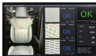
Automated adjudication and labor saving by introducing AI technology to seat appearance and shape inspections (Seating Business)
