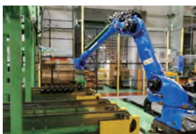
Automatic conveyance and electric sintering treatment by robots for realizing labor and energy savings (Suspension Spring Business)
