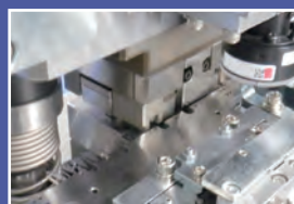
Stamping process for HDD suspensions using high-precision dies
