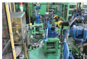
Automatic conveyance and electric sintering treatment by robots for realizing labor and energy savings (Suspension Spring Business)
