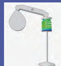
Computer simulation to visualize the behavior of valve springs when driven at high speeds ▶
