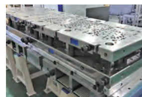
Press work using advanced die design technology (Precision Spring Business)
